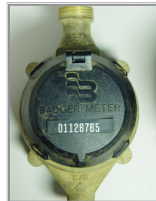
The meter number is located on the lid of the meter
